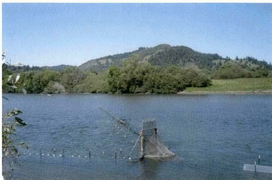
Figure 5. The Estuary fyke net juvenile salmonid video monitoring system located near the town of Duncans Mills.
